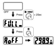
Press "Power" button, and during the LCD shows battery capacity, press "backlight" button until the LCD shows "AoFF" to disable Auto Power Off Function.
